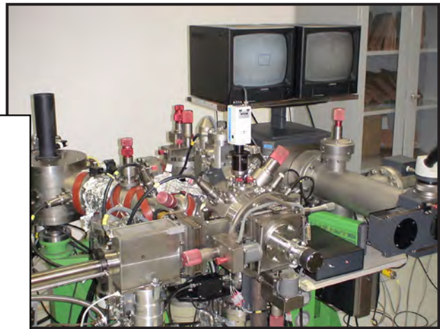
Modified Cameca 4f with 4" Sample Intro System
