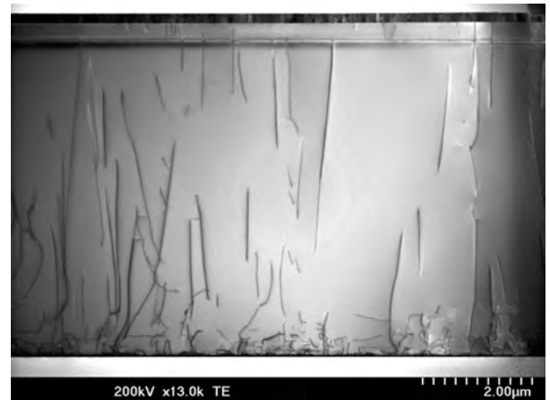
Figure 2: STEM bright field of the identical sample as in Figure 1 showing simplified and more uniform contrast.
